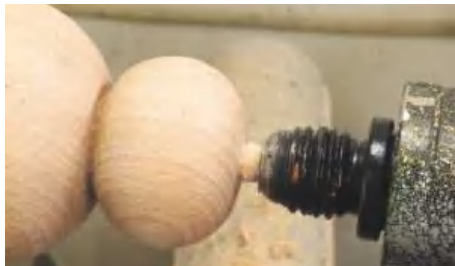
▲ Pic.5 The waste at the tailstock end doesn't need to be taken down any lower than that. The waste can then be cut off with a saw
